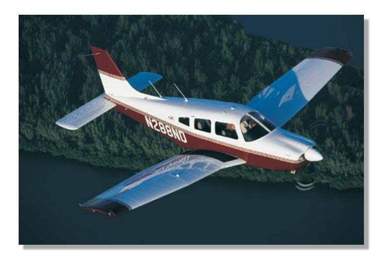
But Cherokees have disadvantages, too. You've got to be nimble to crawl around under that low wing to sample fuel, and examine the bottom of the wing. An apparent Cherokee advantage, the ease with which it lands, actually can cause problems when you start flying other kinds of airplanes
